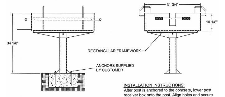
NOTE : CUSTOMER TO PROVIDE CONCRETE ( RECOMMENDED )
